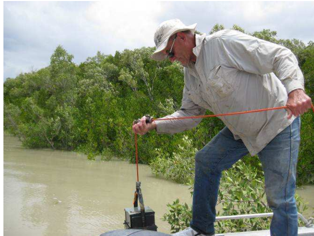
Figure 2-2: Birge-Eckman grab sampler being lowered from the boat (Photo: ALS Water Sciences)
