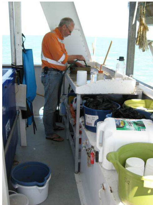
Figure 2-3: Benthic fauna samples being washed through a 600 \mu m sieve aboard the mother ship (Photo; ALS Water Sciences)
